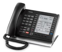
9-line Backlit LCD 20 programmable buttons and LCD key labels
