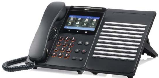
DT930S touch panel + 60-line DSS
